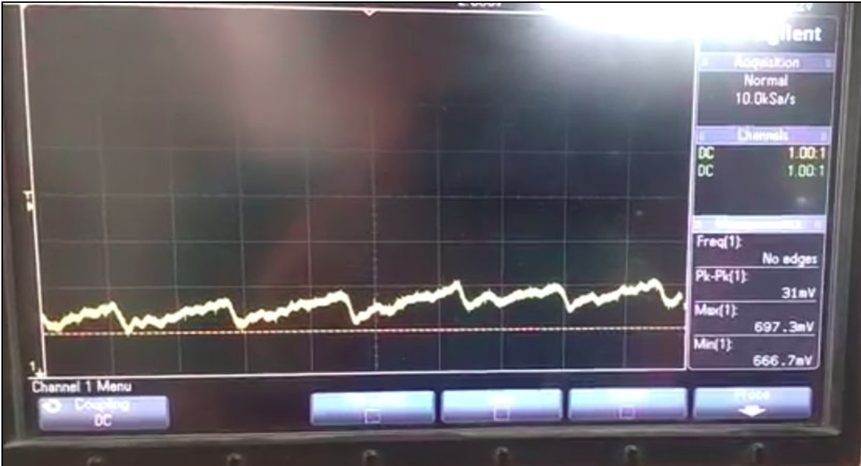
Figure 4.1 : PPG Signal with low pk-pk (~ 31 mV) on oscilloscope
