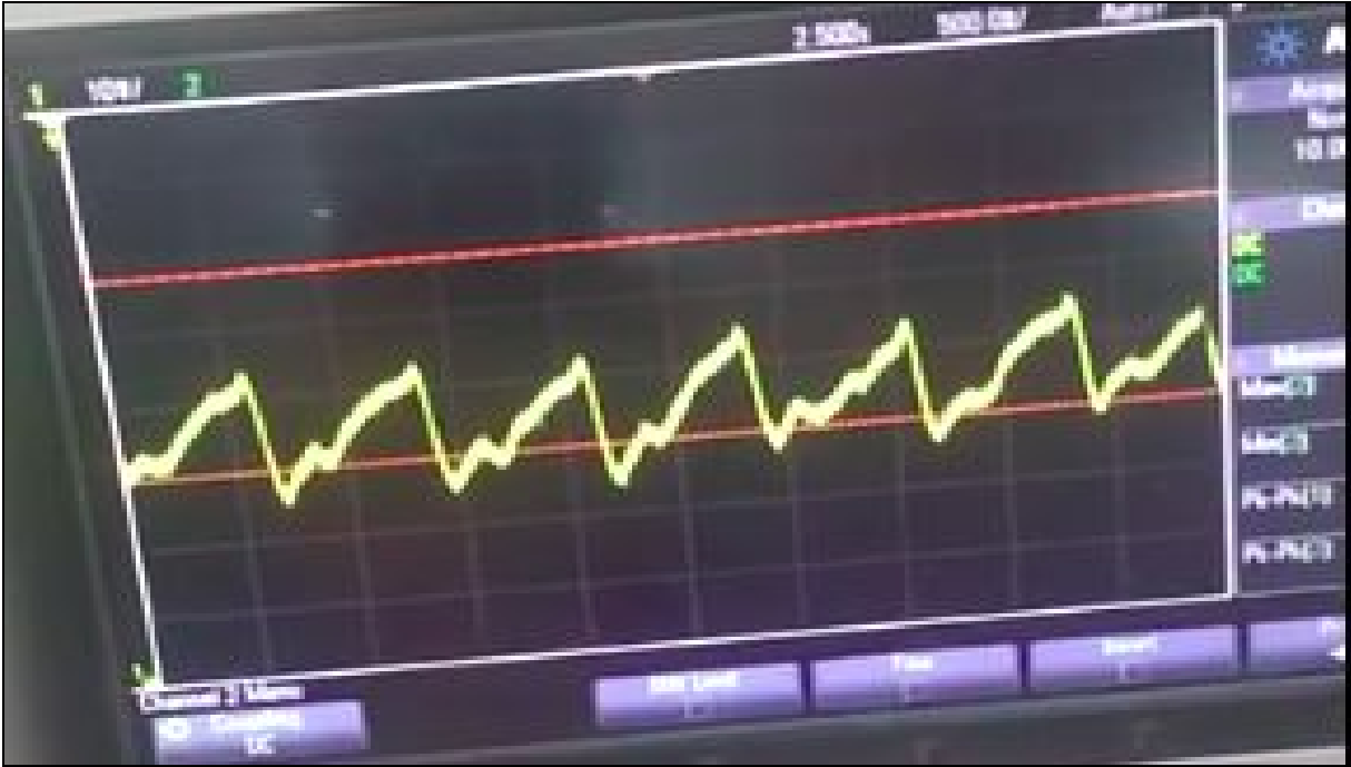
Figure 4.2 : PPG signal amplified to pk-pk ~ 1V on oscilloscope
