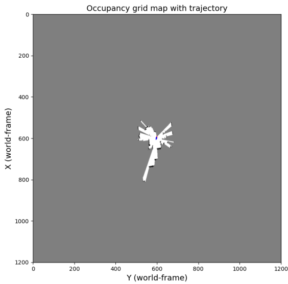
Figure 9. Figure showing map during PF-SLAM with 100 particles, \sigma_v = 0.5 , \sigma_\omega = 0.05 , trajectory step 500
