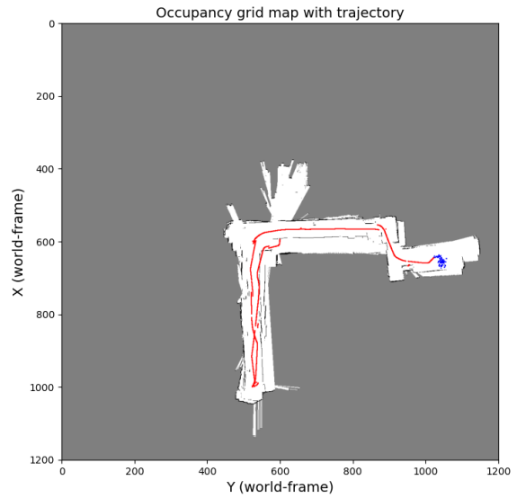
Figure 72. Figure showing map during PF-SLAM with 100 particles, \sigma_v = 0.5 , \sigma_\omega = 0.05 , trajectory step 3500
