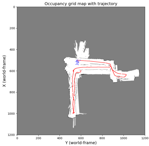
Figure 74. Figure showing map during PF-SLAM with 100 particles, \sigma_v = 0.5 , \sigma_\omega = 0.05 , trajectory step 4500
