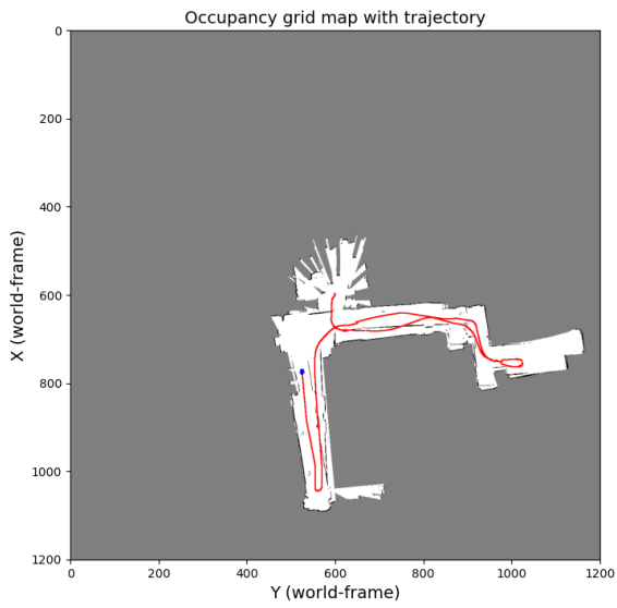
Figure 32. Figure showing map during PF-SLAM with 100 particles, \sigma_v = 0.1 , \sigma_\omega = 0.01 , trajectory step 4000
