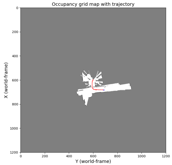
Figure 26. Figure showing map during PF-SLAM with 100 particles, \sigma_v = 0.1, \sigma_\omega = 0.01 , trajectory step 1000
