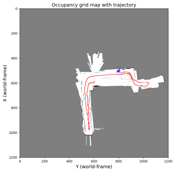
Figure 89. Figure showing map during PF-SLAM with 100 particles, \sigma_v = 0.5 , \sigma_\omega = 0.1 , trajectory step 4000
